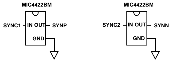
FIGURE 22B. NON-INVERTING DRIVERS
